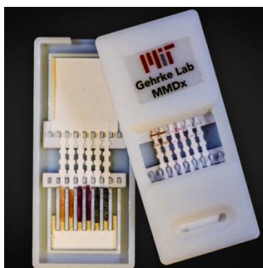
Fig: A new paper diagnostic device can detect Ebola and other viral hemorrhagic fevers in about 10 minutes. The device has silver nanoparticles of different colors that indicate different diseases. On the left is the unused device, opened to reveal the contents inside. On the right, the device has been used for diagnosis; the colored bands show positive tests
